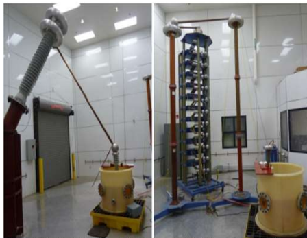
Figure 3: AC w/ PD test set (left), Negative lightning impulse and switching surge test set (right)
