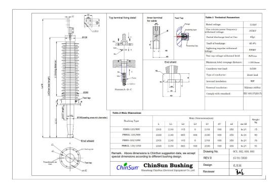
Drawing-transformer bushing-123kV\_silicone rubber-DL-ChinSun
