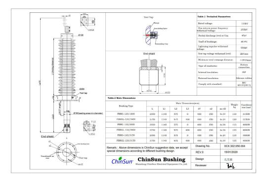
Drawing-transformer bushing-123kV\_Silicone rubber-BC-ChinSun
