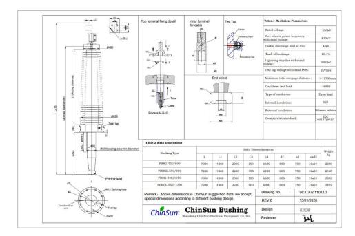
Drawing-transformer bushing-550kV\_silicone rubber-DL-ChinSun
