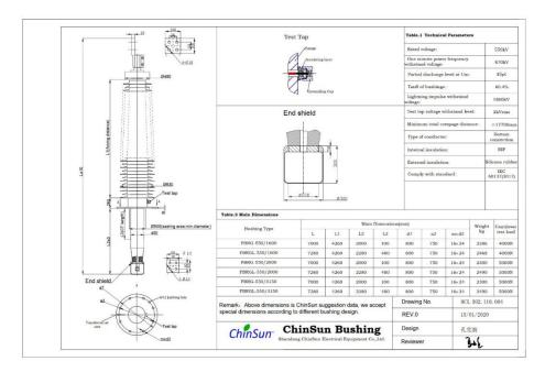
Drawing-transformer bushing-550kV silicone rubber-BC-ChinSun
