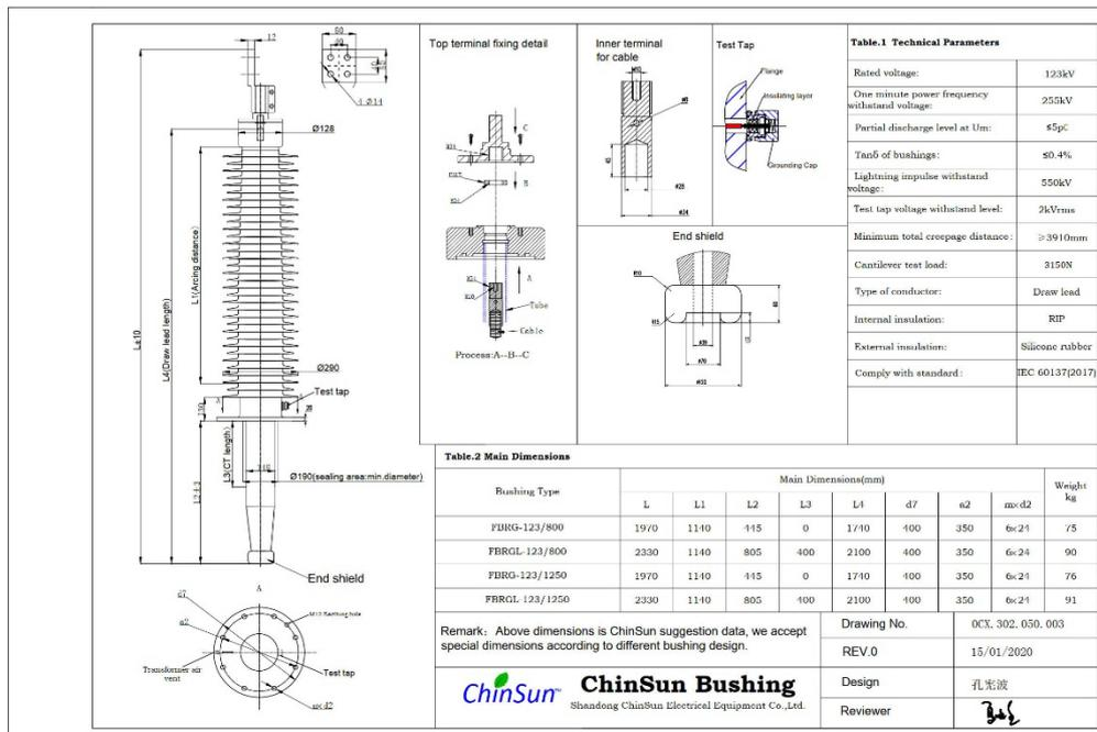
Drawing-transformer bushing-123kV\_silicone rubber-DL-ChinSun
