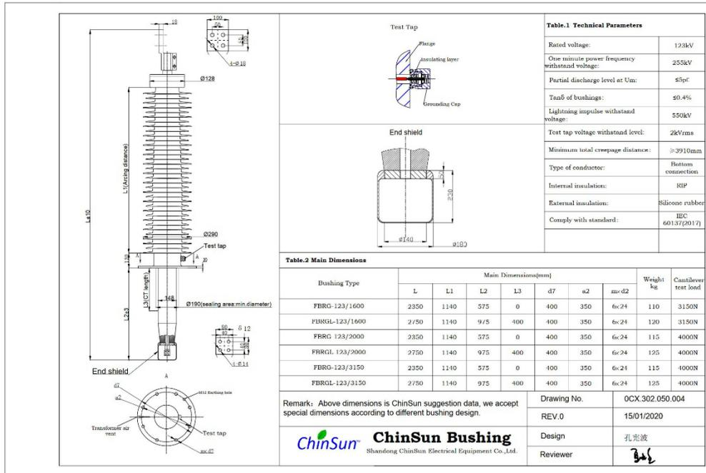
Drawing-transformer bushing-123kV\_Silicone rubber-BC-ChinSun
